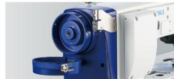
In a situation where the power is on, the handwheel cover with the open / close sensor prevents the sewing machine from starting suddenly. In addition, the cover prevents thread and material from being caught in the handwheel during sewing.
