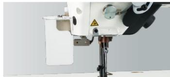
The eye guard prevents a broken needle from flying off. If the eye guard is open, the sewing machine cannot be started. As a result, the sewing machine will not start up unexpectedly even if the operator forgets to turn the power off.
