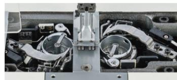
The sewing machine will not start if the throat plate is open. This prevents the material from being caught in the hook during sewing.
