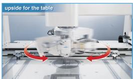
The head turning mechanism at the upside and underside of the table rotates in the sewing direction.
